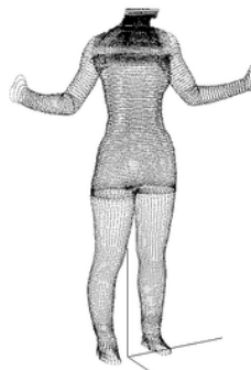
Figure 4. 3D cloud of coordinate points of a virtual model of the subject scanned
