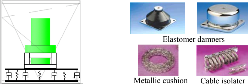
Figure 5. Presentation of the concept with a transportation pallet working principle
