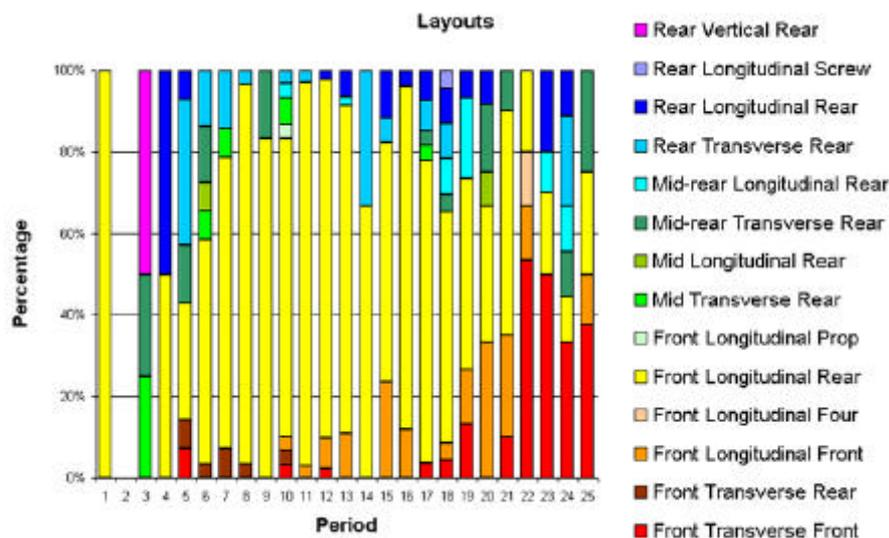
Figure 3: Engine position, orientation and drive for periods.
