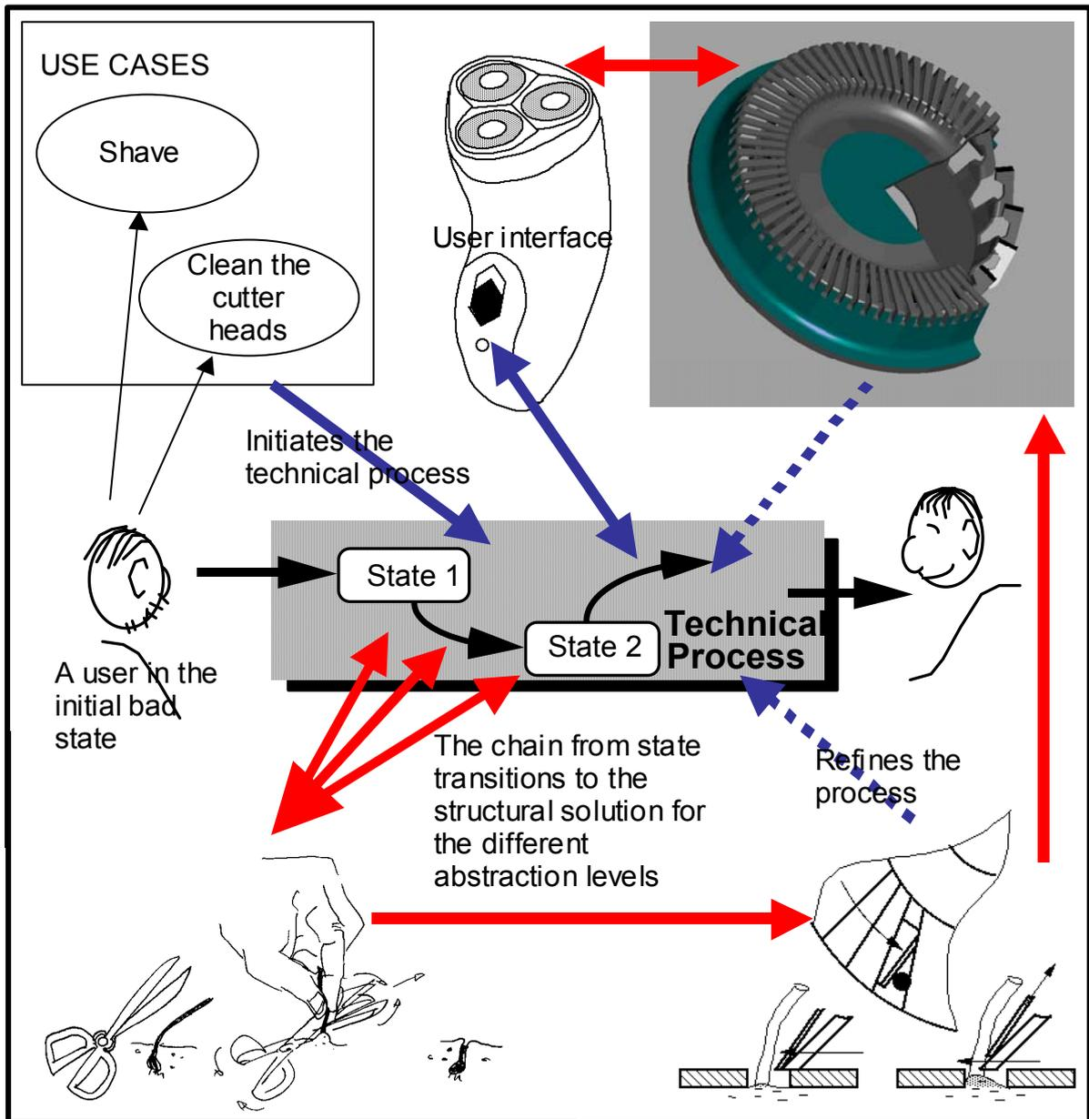
Figure 4. Design data is maintained and managed in the state transition model of the technical process.
