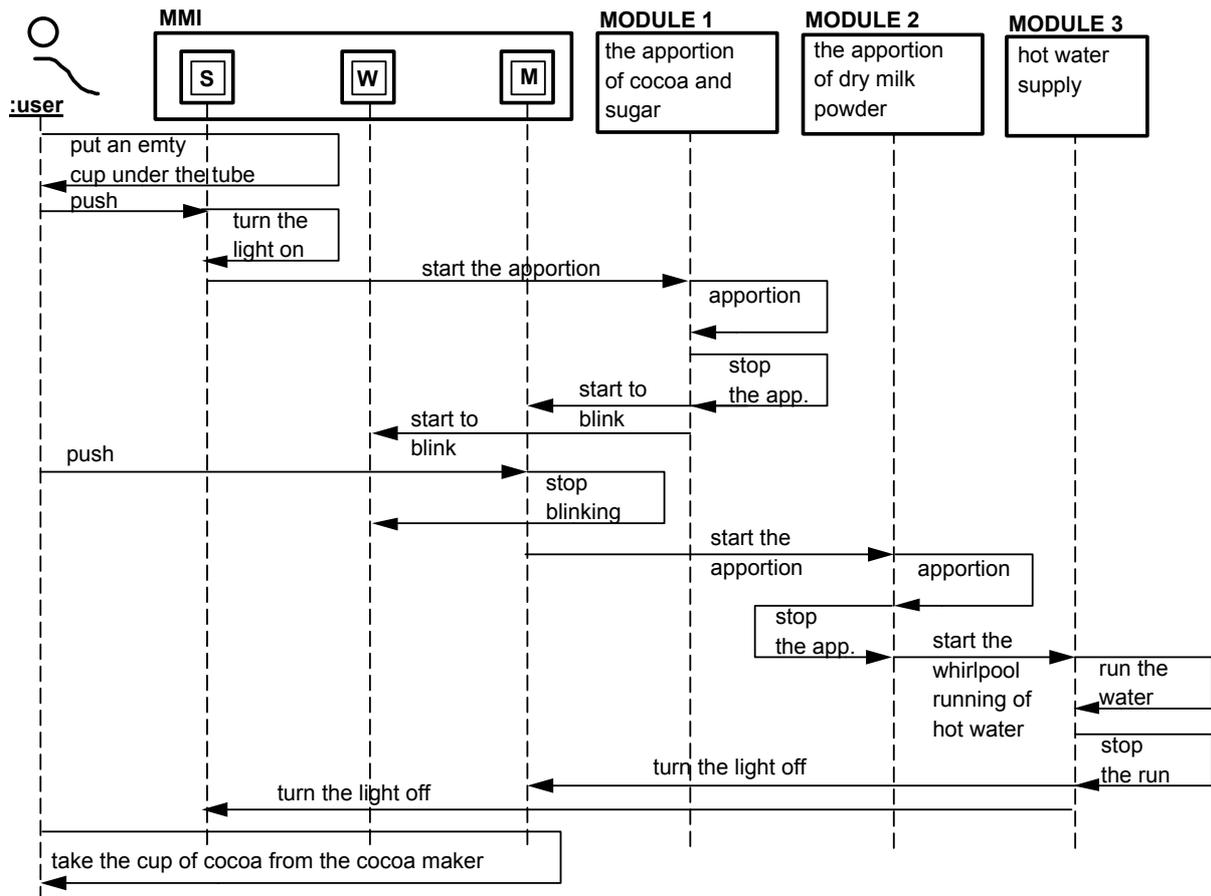
Figure 9. The sequence diagram for making a cup of cocoa with milk.
