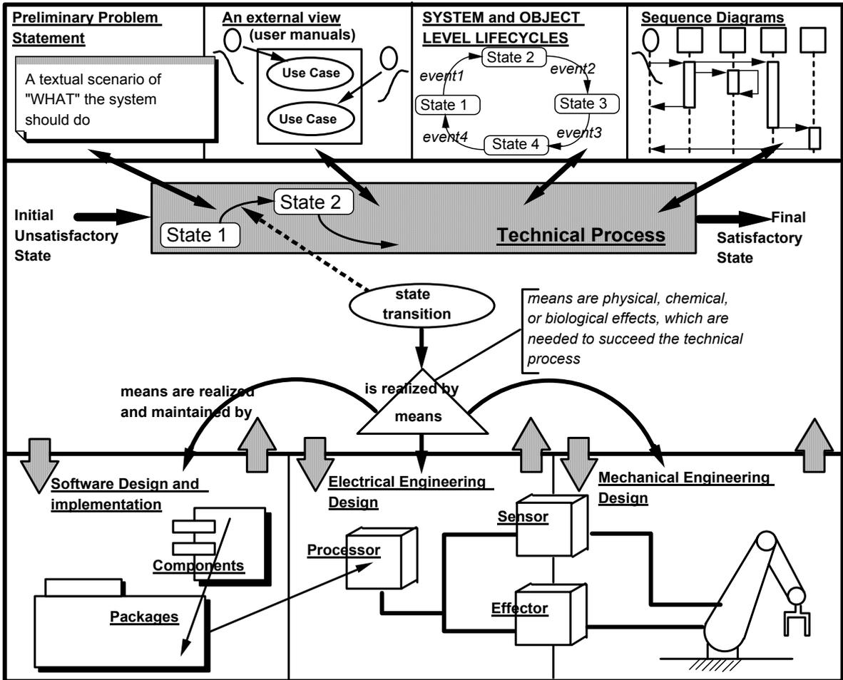
Figure 5. The layered design process of a mechatronic product.
