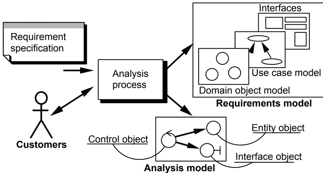
Figure 2. The OOA-process for system modelling by Ivar Jacobson [7].
