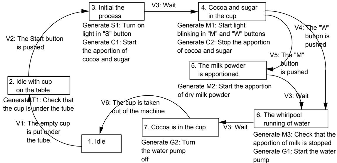
Figure 8. State model of the cocoa making process.
