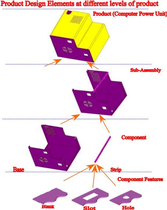
Figure 4: Product Design Elements (PDE) at different levels of a sheet metal product
