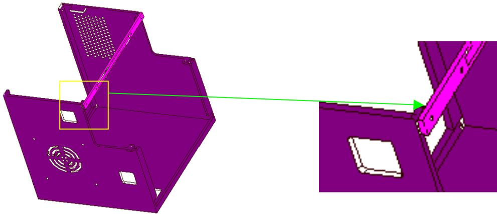
Figure 5 Assembly of Base and Strip in Computer Power Unit
