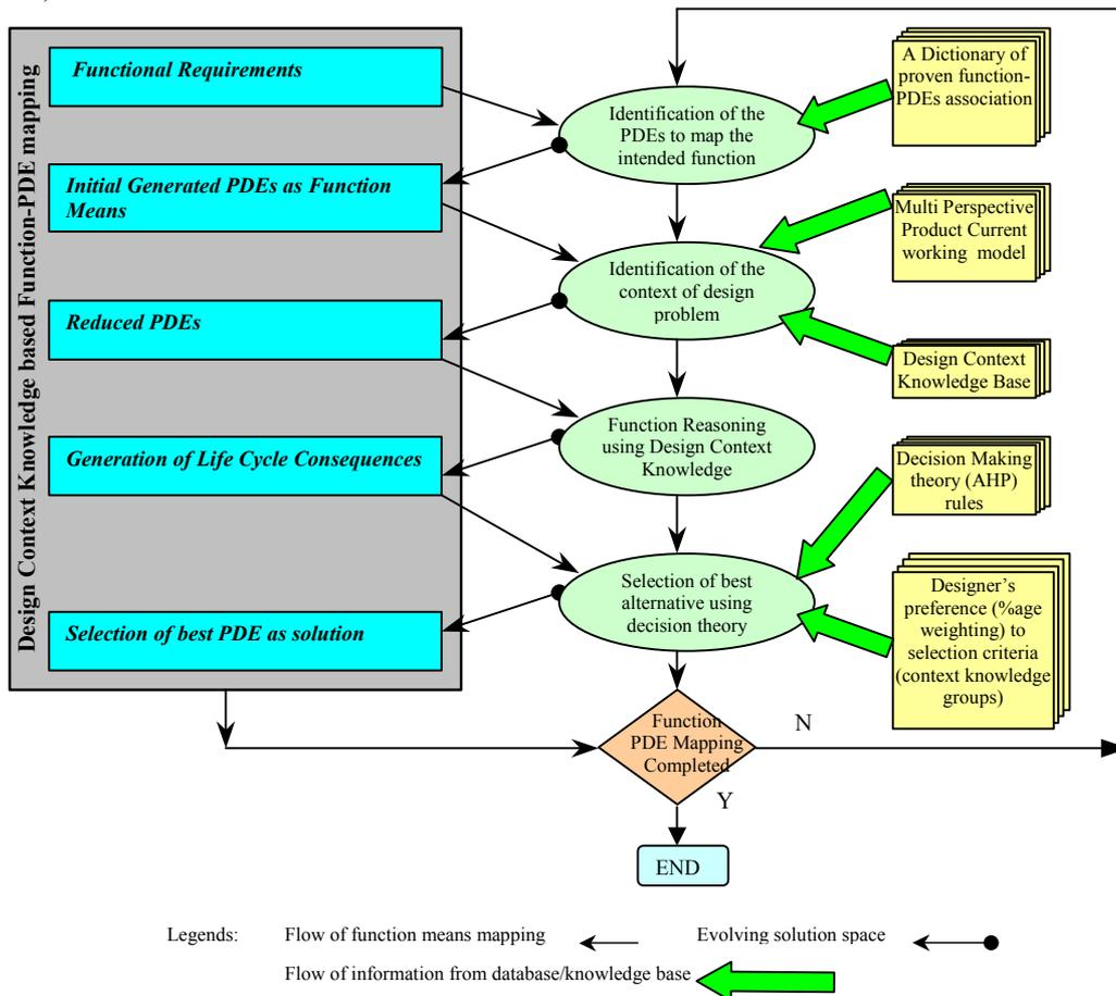
Figure 3. Function to PDE(s) mapping process model
