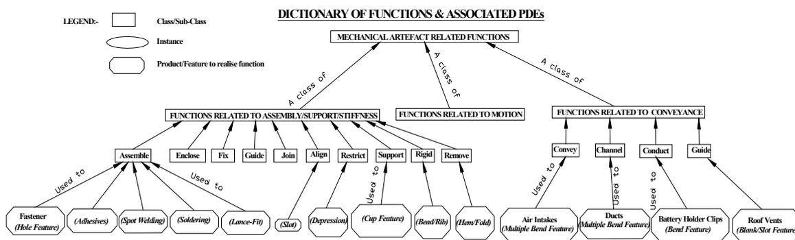
Figure 2. Some functions and associated PDEs from dictionary
