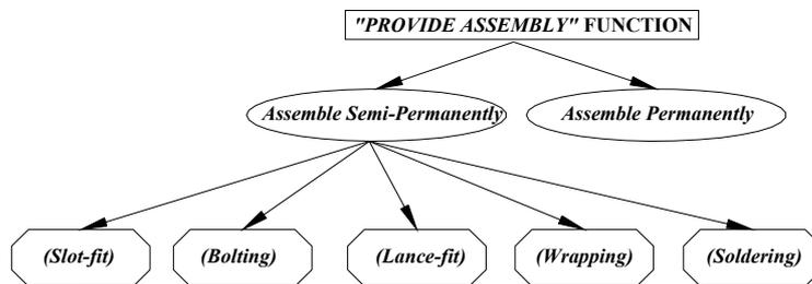
Figure 6 Function decomposition and initial PDEs/solutions to fulfil “*Semi-Permanent Assembly*” function
