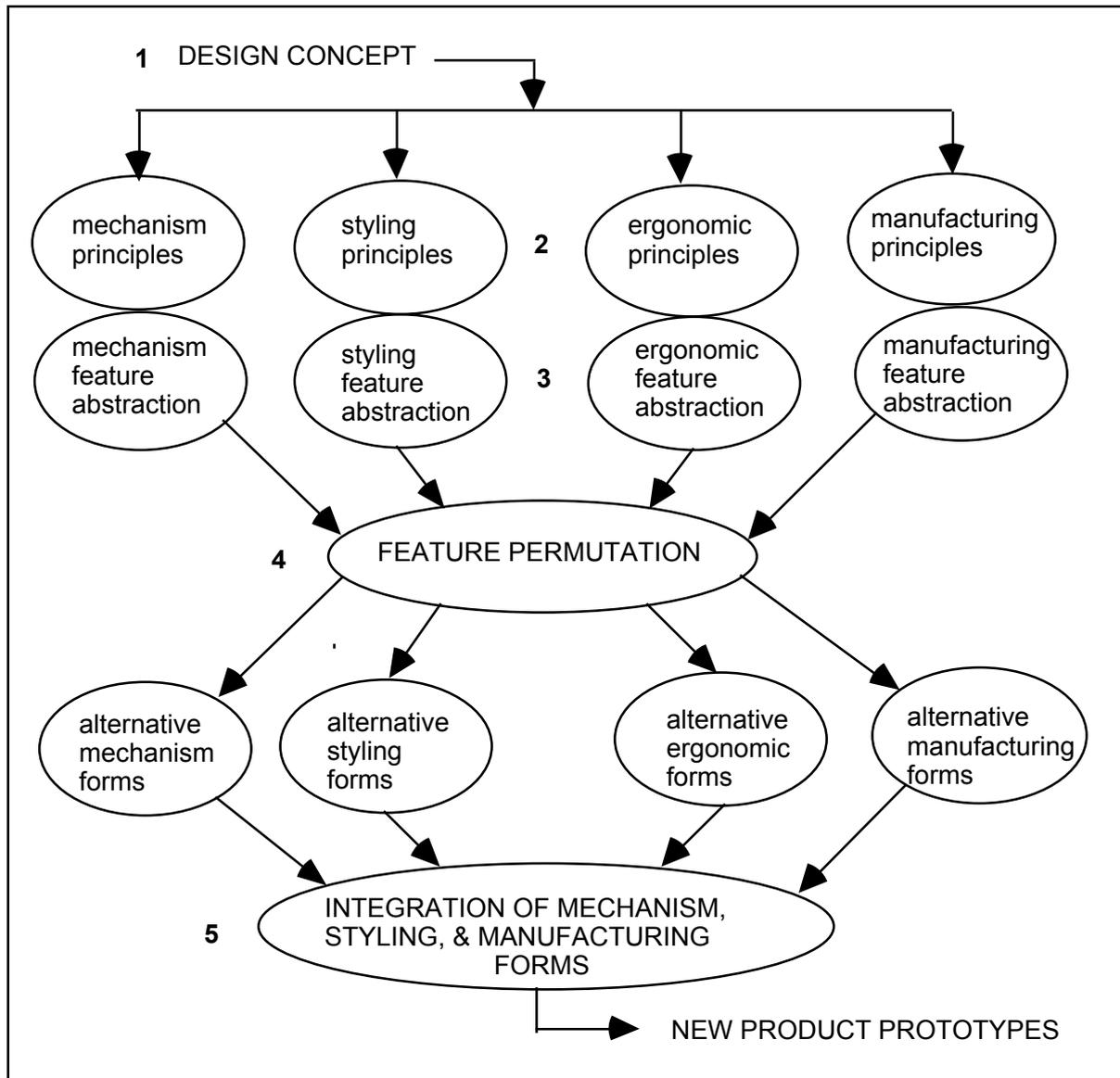
Figure 6. A structured design process
