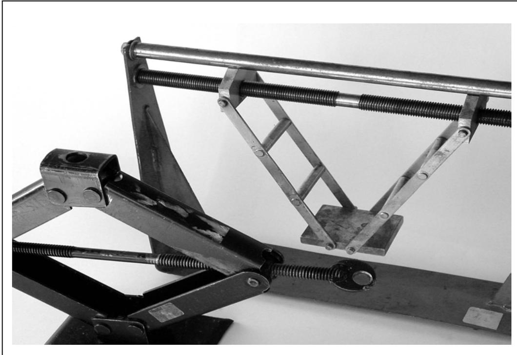
Figure 4. The proprietary scissor jack used as a source of ideas
