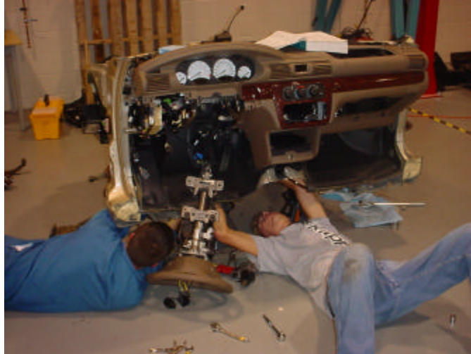
Figure 5. Automotive Engineering Project Room at Windsor. Vehicle manufacturers have provided a number of products which students use for projects. The team above is disassembling the front-end of a 2001 Chrysler Sebring automobile to examine the HVAC systems and front suspension and brake components. The engine and transaxle of the Sebring have already been the subject of another project.
