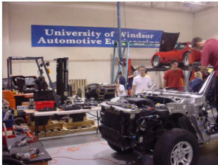
Figure 6. Automotive Engineering Project Room at Windsor. The team depicted above is partially disassembling a 2002 Dodge Dakota pick-up truck to create an operable instructional aid that can be used to examine how modern vehicles are built and how the various parts function together. The vehicle hoist in the background is used to allow students to safely examine various types of vehicles and learn how they are constructed.
