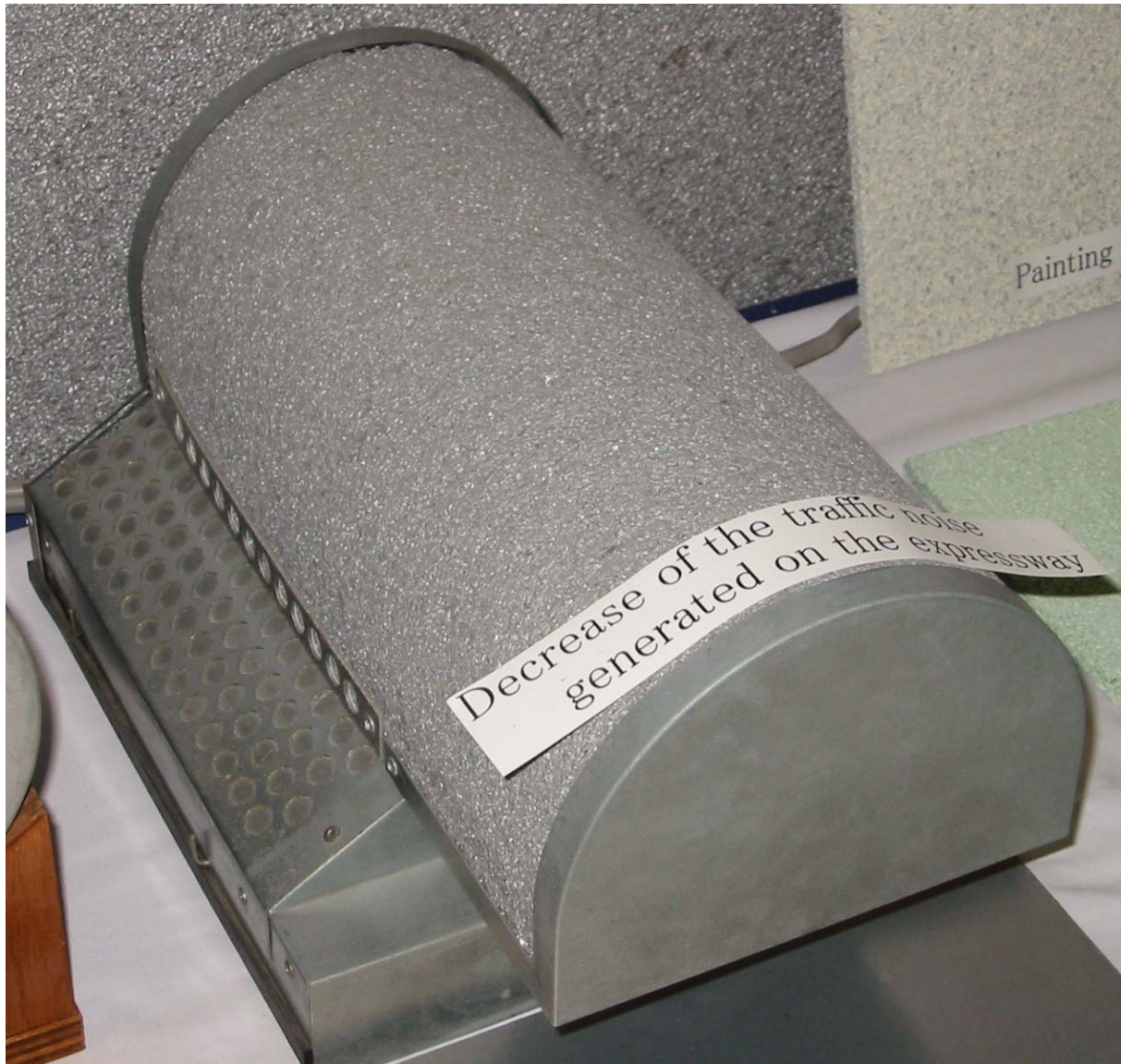
Figure 4. Example of application – sound absorber for expressway
