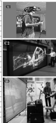
Figure 3 Combinations C1, C2 and C3 consist respectively of HDM coupled with a common mouse, a large volume display provided with stereo imaging and an optic tracking system and a similar display with a point-based device for simulating assembly operations
