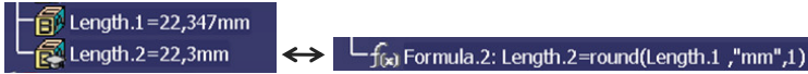
Figure 8: mathematical function round() to round up a length parameter with 1 digit after comma
