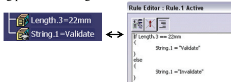
Figure 9: KWA rule - the value of a string parameter is defined using a conditional instruction
