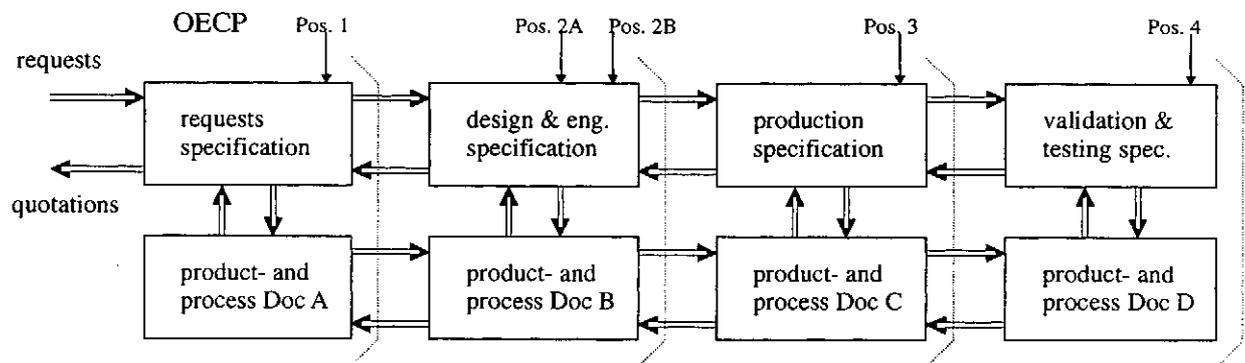
Figure 7. The quotation and estimation trajet: introduction of the Order Entry Calculation Point (OECP).
