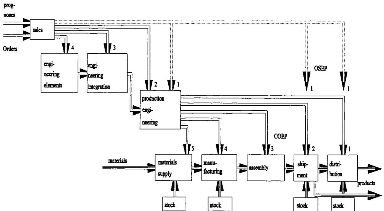
Figure 4. Different positions of COEP and OSEP in the sales, engineering and manufacturing process
