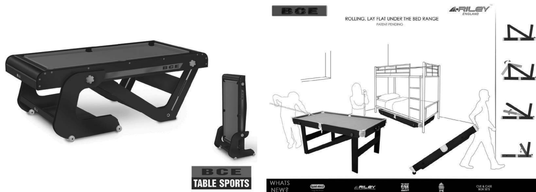
Figure 1. BCE Table Sports Design and Folding Mechanism
