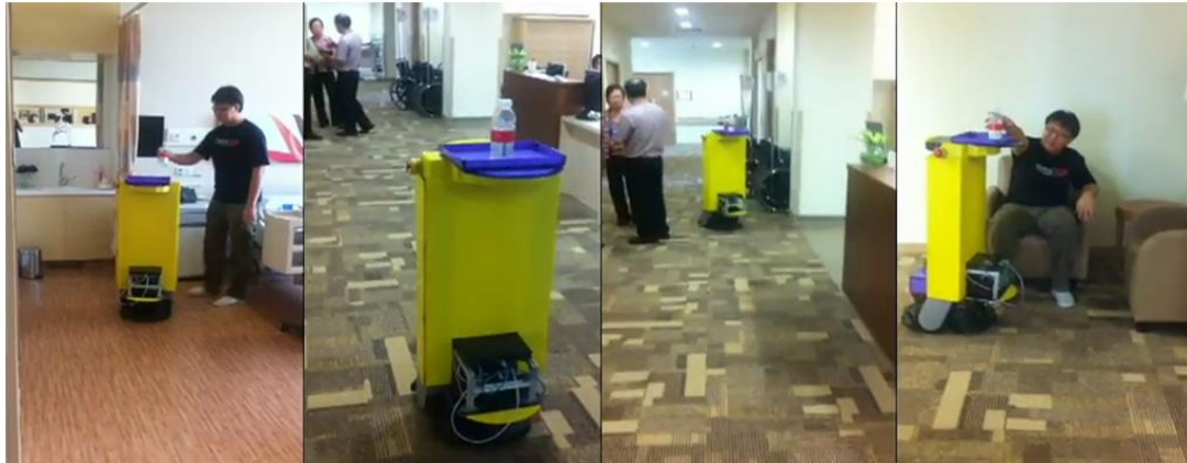
Figure 1. Feasibility study involving the service robot for specimen delivery task at Singapore based hospital. The robot platform is an Adept PeopleBot.
