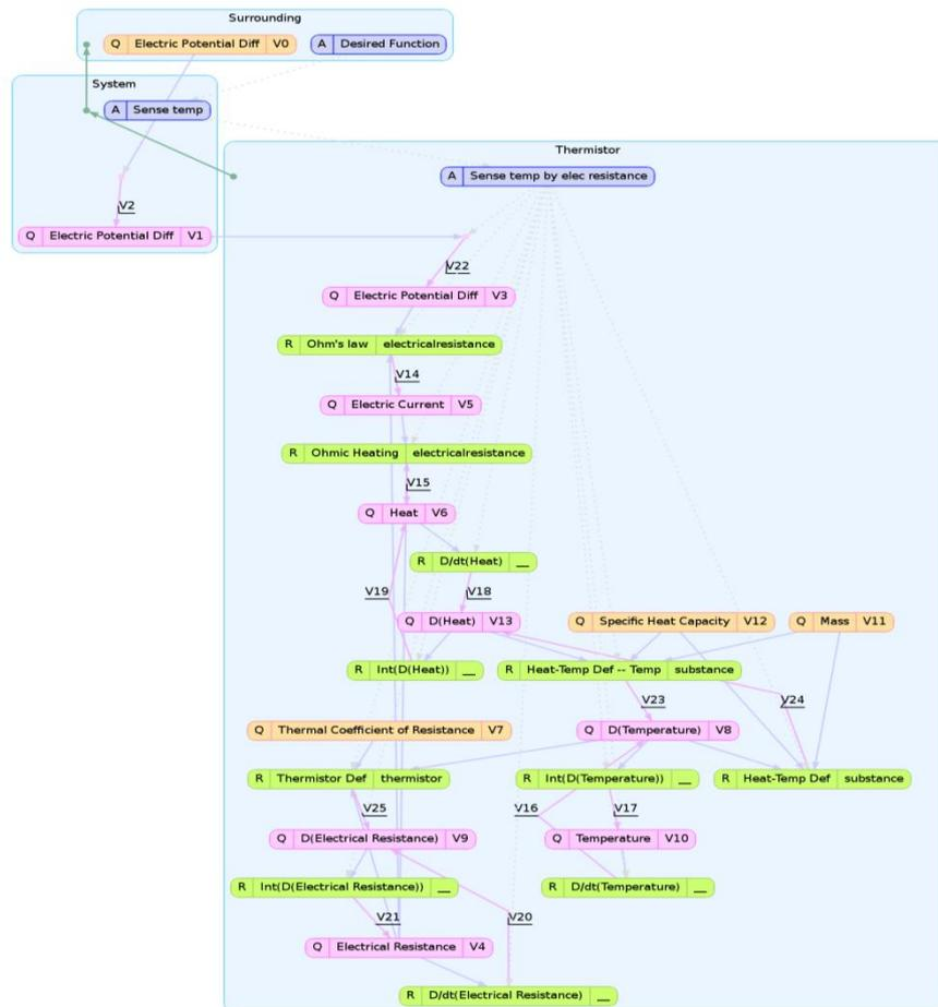
Figure 2: SAPPPhIRE-lite model of Thermistor (Temperature dependent resistor). Quantities are indicated by the label ‘Q’ and relations by ‘R’. The quantities and relations form a network.
