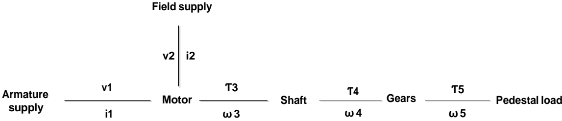
Fig 5. Word bond graph for the Antenna system. Where \tau = torque, \omega = angular velocity, v = voltage, i = current.
