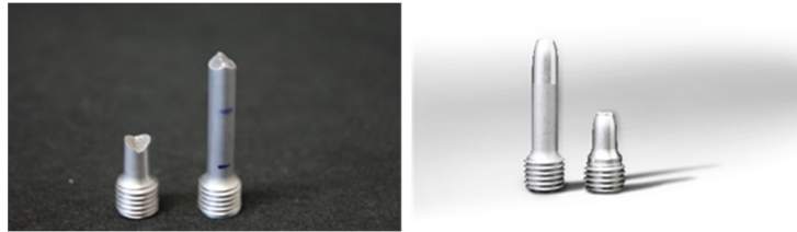
Figure 6. Fracture type and position of a specimen (powder only) (b) Fracture type and position of a specimen (cast basic structure and powder)
