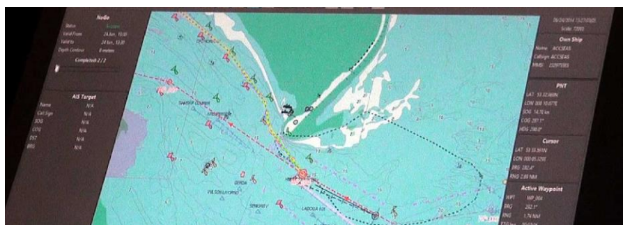
Figure 5. The yellow segment has been sent to the ship from the VTS and recommends using the Northern channel.
