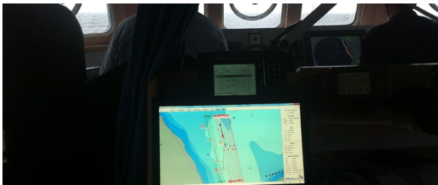
Figure 6. Search patterns for this rescue boat is transmitted directly to the onboard chart system.
