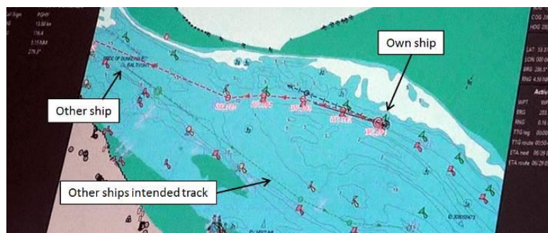
Figure 4. By right-clicking on another ship and selecting “show intended track” other ship’s intentions can be visualised.
