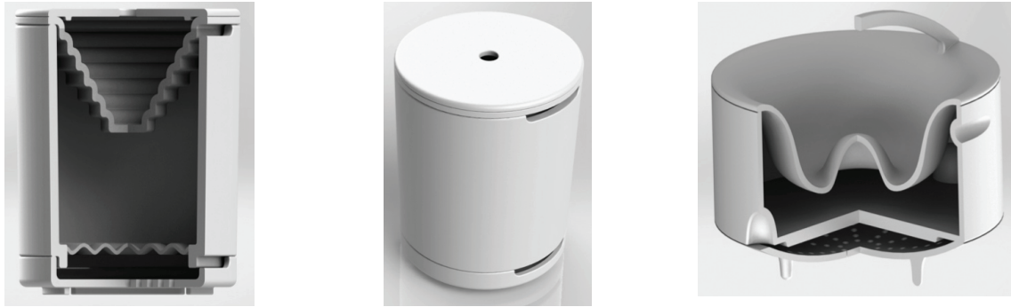
Figures 15-17. Renders of final ceramic filter design for initial tests in Malawi
