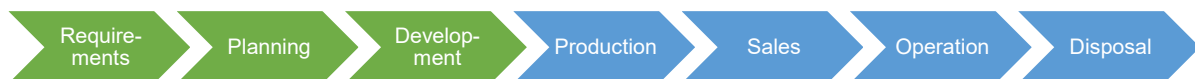
Figure 1: The steps of the PDP in green are a subset of the PLC in blue and green [6].
