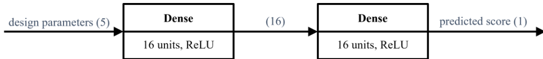
Figure 5. Base architecture for neural networks of the ensemble of the Active Learning approach.
